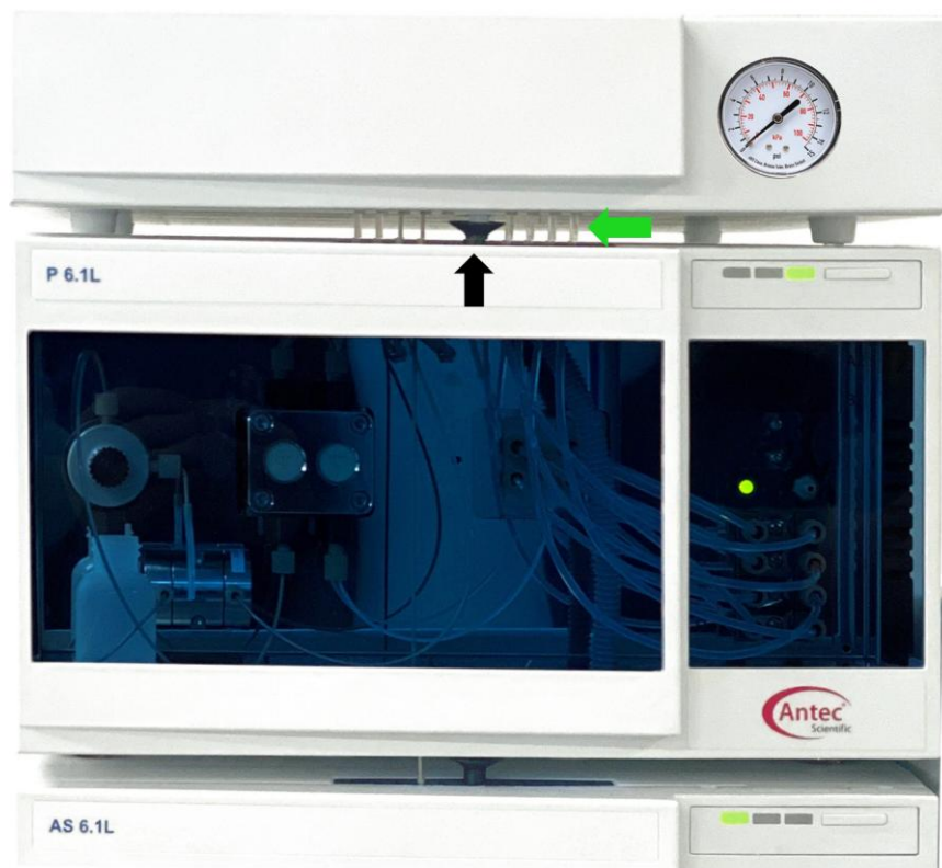
Fig. 3. ALEXYS HPLC system stack with ET 210 on top.
