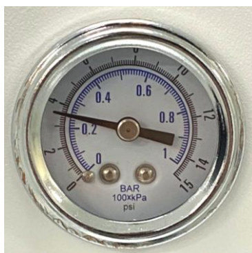
Fig. 7. ET 210 manometer: scale in PSI (0 – 15 psi) and bar (0 – 1 bar).
